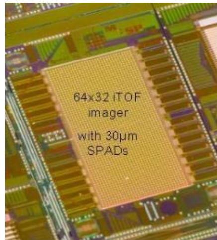
Fig. 2: Array chip containing the 64x32 pixels with 2048 SPAD detectors.
