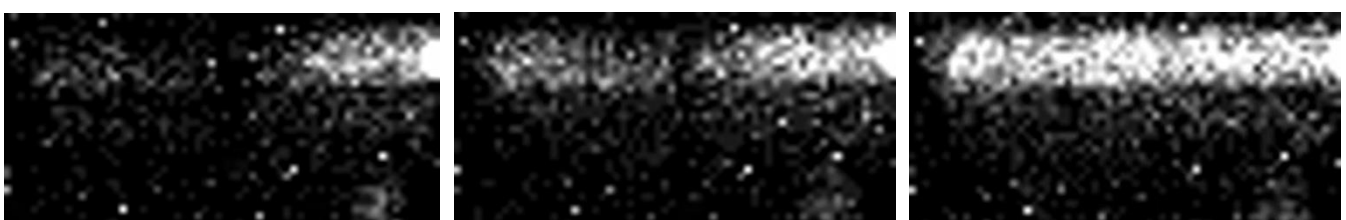
Fig. 12. Propagation of a laser pulse in an acrylic slab, as seen by the SPAD camera. Each frame is taken each 80 ps, for an equivalent frame rate of 12.5 Gfps!
