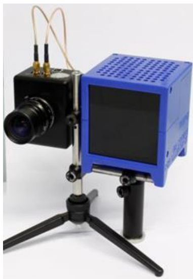
Fig. 8: Left: 64x32 SPAD camera with 3W laser illuminator at 808nm, for 3D ranging. Right: Matlab Graphic User Interface.
