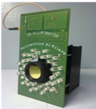
First Prototype of MiSPiA 3D camera (imager plus illuminator) for the indirect TOF (Time-of-Flight) laboratory tests.
